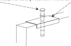
**4.** Attach the Strike Plate as shown on back of door, opposite side of pivot brackets. Use screws provided.
