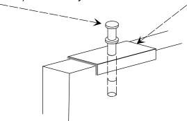
**4.** Attach the Strike Plate as shown on back of door, opposite side of pivot brackets. Use screws provided.
